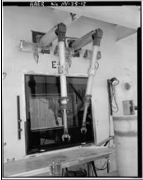
Abb.2 Manipulatorarme in der Hot Bay von Area 25, Nevada Test Side 1962-1973
